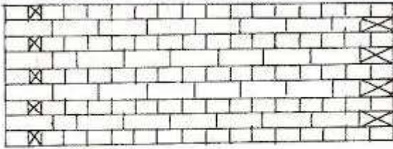
Elevation of wall in English cross-bond.
