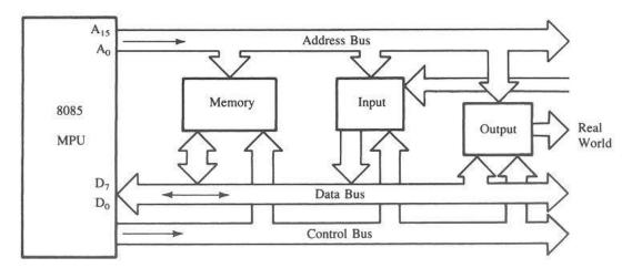
Figure 1-Bus structure of 8085
