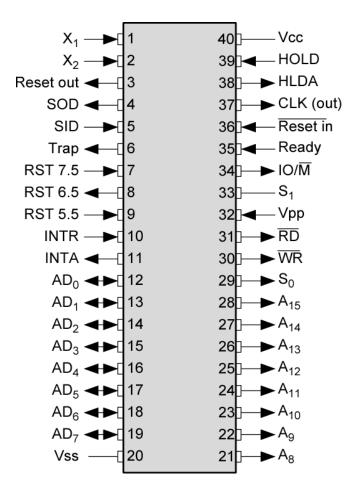
Figure 5-Pin diagram of 8085
