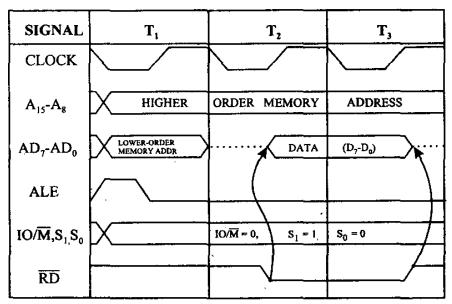
**Timing Diagram for Memory Read Machine Cycle**
