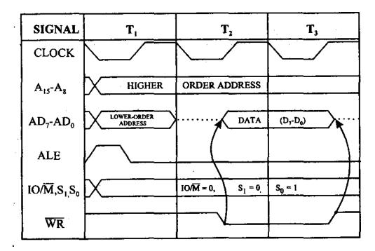
**Timing Diagram For Memory Write Machine Cycle**
