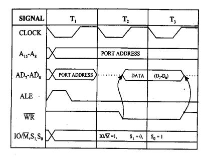
Timing Diagram for I/O Write Machine Cycle
