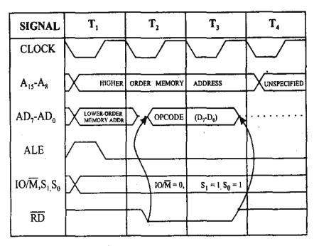
Timing Diagram for Opcode Fetch Machine Cycle Memory Read Machine Cycle of 8085:
