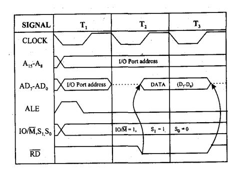
Timing Diagram for I/O Read Machine Cycle
