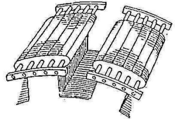
(a) Continuous damper (b) Non-continuous damper
