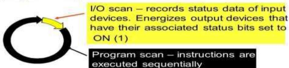
Because the inputs can change at any time, the PLC must carry on this process continuously.
