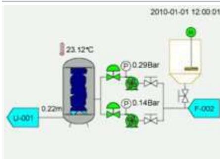
Typical SCADA mimic shown as an animation. For process plant, these are based upon the piping and instrumentation diagram.
