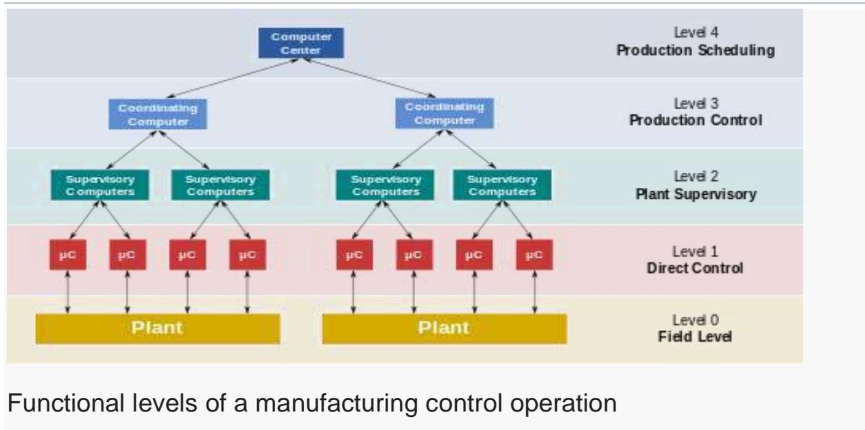
Functional levels of a manufacturing control operation
