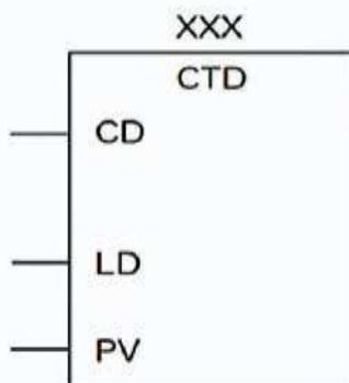
Each time the input CD turns ON the counter decrement one from the preset value. Whenever LD (load) input becomes high then the preset value is reloaded to the counter from the current value.
