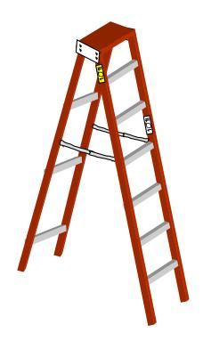
Ladders used around electrical hazards must have non-conductive side rails. Ladders with non-conductive side rails that are contaminated with paint, greases or other coatings may no longer be non-conductive. Check them out.
