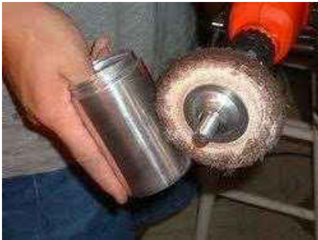
Schematics of the buffing operation.
